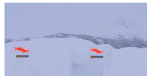
DroneOptID Software detecting and classifying multiple drones against arctic backdrop. Red overlay represents pixels identified as 'drone object' tracked by the software.
