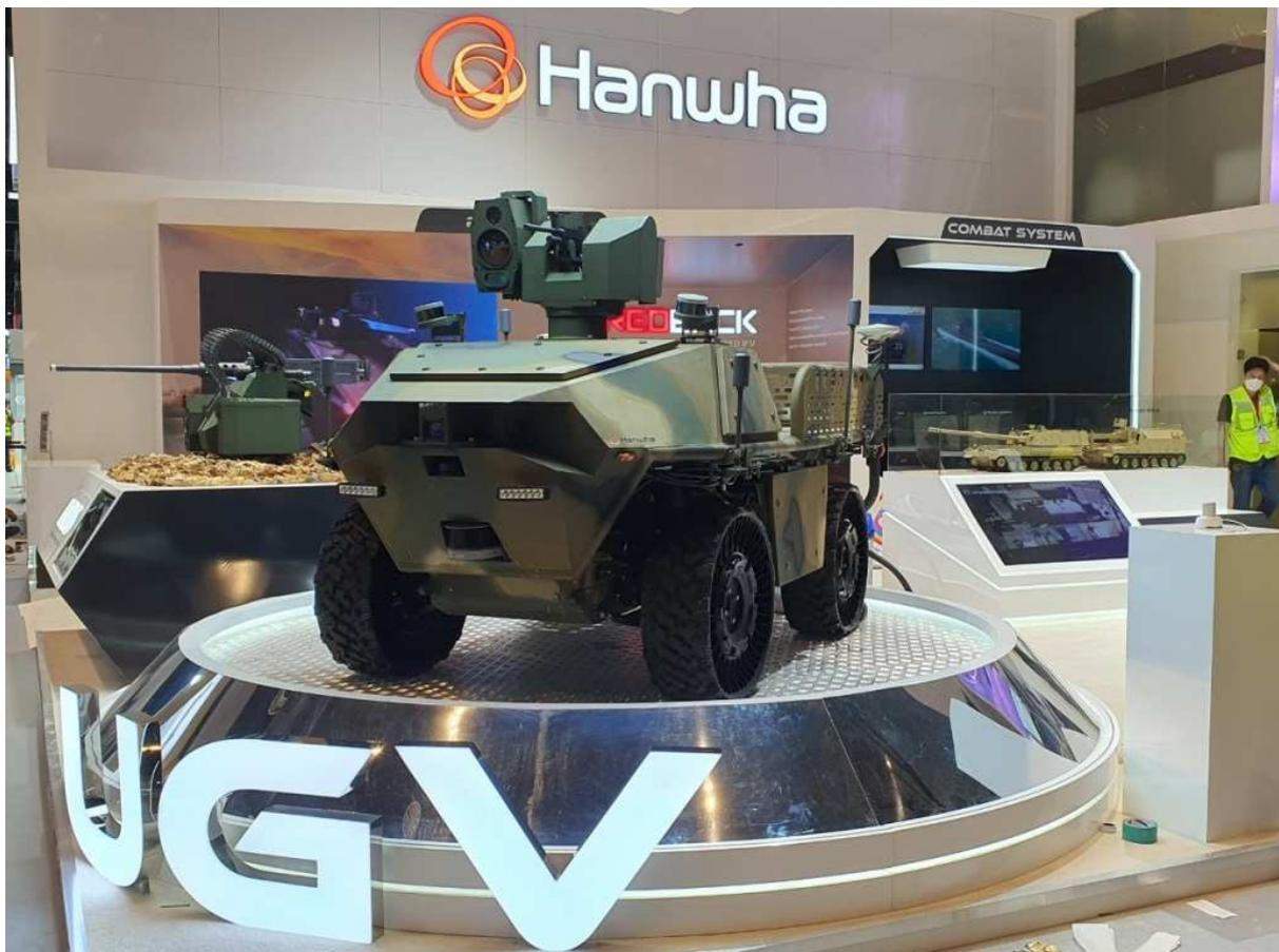
The 4x4 vehicle operates on electricity and can move at a top speed of 30 km/h on paved roads. On the battlefield, the 1.5-ton vehicle is operated either remotely or autonomously to carry out various missions, such as surveillance, logistics transport, evacuation of casualties and combat engagement.
